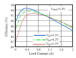
Figure 2. Efficiency VS Load Current
