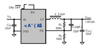
Figure 1. Basic Application Circuit
