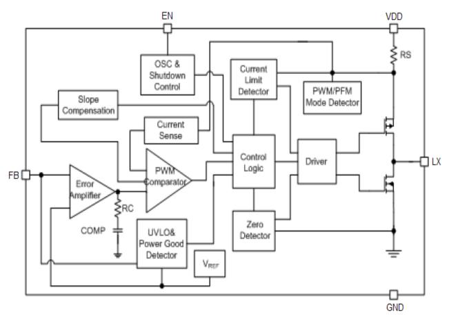
Figure 3. HM3420 Block Diagram
