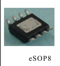
The PWM control circuit is able to adjust the duty ratio linearly from 0 to 100%. An enable function, an over current protection function is built inside. An internal compensation block is built in to minimize external component count.
