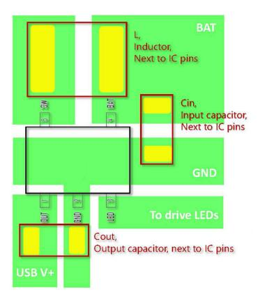
Please have the power devices placed just next to the IC pins so that the power traces are kept the shortest way to achieve a good performance of HM5909.
