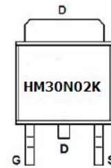
Marking and pin assignment
