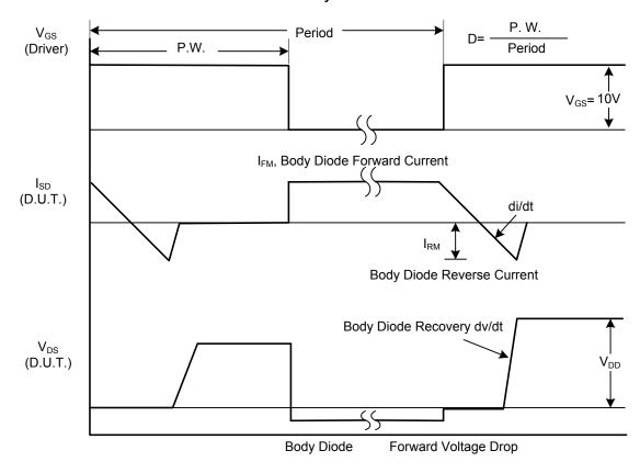
Peak Diode Recovery dv/dt Waveforms
