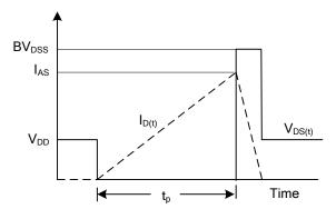
**Unclamped Inductive Switching Waveforms**
