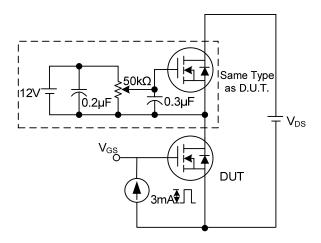
Gate Charge Test Circuit
