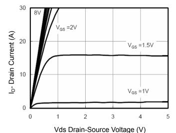
**Figure 5 Output Characteristics**
