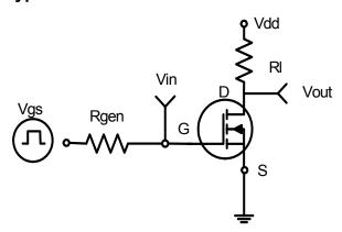
**Figure 1:Switching Test Circuit**
