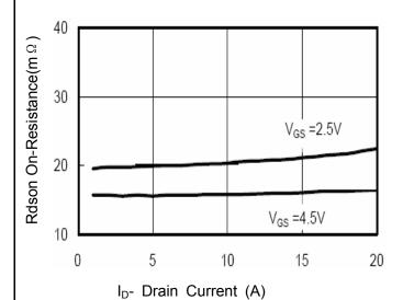
Figure 6 Drain-Source On-Resistance
