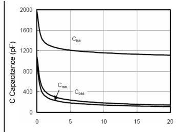
Vds Drain-Source Voltage (V)
