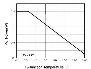
Figure 3 Power Dissipation
