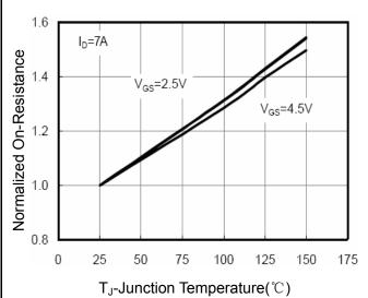
Figure 8 Drain-Source On-Resistance
