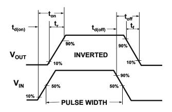
Figure 2:Switching Waveforms
