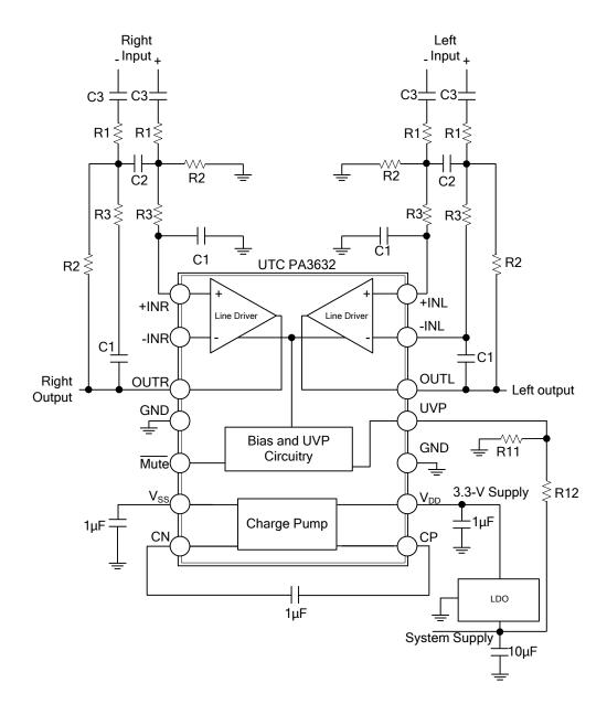
R1 =  $15k\Omega$ , R2 =  $30k\Omega$ , R3 =  $43k\Omega$ , C1 = 47pF, C2 = 180pF Differential-input, single-ended output, second-order filter
