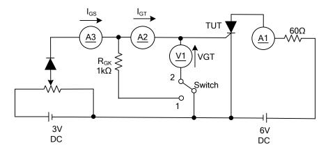
Switch 1:  $I_{GT}$  Measurement Switch 2:  $V_{GT}$  Measurement
