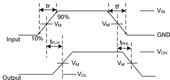
Notes: 1.  $V_{OL}$  and  $V_{OH}$  are typical output drop that occur with the output load.
