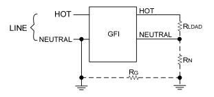
Normal Fault plus Grounded Neutral fault: The combination of the normal fault and the grounded neutral fault, as shown by the dashed lines.
