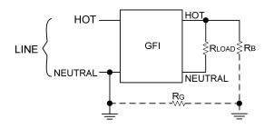
Grounded Neutral Fault: An unintentional electrical path between the load terminal of the neutral line and the ground, as shown by the dashed lines.
