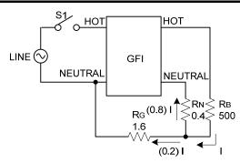
UL943 specifies ≤25 ms average trip time under these conditions. Calculation of Ct based upon charging currents due to normal fault only is as follows:
