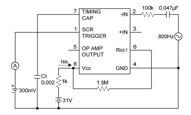
FIGURE 1.Normal Fault Sensitivity Test Circuit
