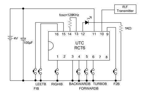
UTC **RCT6** output pin (SO) has an inverted phase with UTC **RCR6C** input (SI). If UTC **RCT6** is connected without using a R<sub>F</sub> module, an inverter has to be inserted between this 2 pins.
