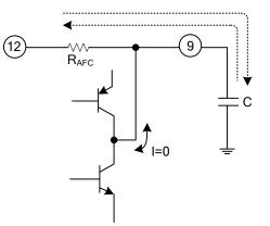
As can be seen from the above circuit diagrams, the time constant during detuning is determined by the internal PNP resistance, the NPN collector resistance and the capacitance of the externally-mounted capacitor. This time constant is determined by the external resistance RAFC and capacitor
