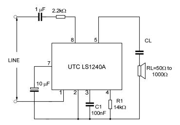
No current limitation is provided on the output stage of UTC **LS1240A**, so a minimum load DC of 50 ohms is advised.
