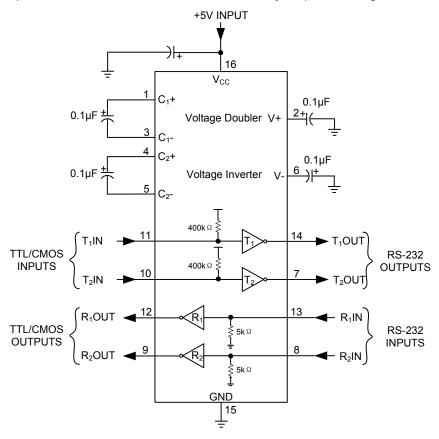
Connecting the capacitor to  $V_{\text{CC}}$  (+5.0V) is recommended.
