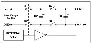
Figure 2 Charge Pump Voltage Inverter
