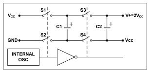
Figure 1 Charge Pump Voltage Doubler
