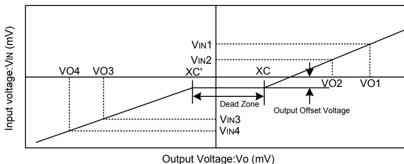
$$* \text{ Voltage Gain } G_{vc(+)} = 20 \log \frac{V_{O1}-V_{O2}}{V_{IN1}-V_{IN2}}$$
