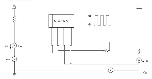
$\label{eq:local_continuous} \text{Measure V}_{\text{CC}}, I_{\text{CC}} \text{ when DO is off.} \quad \text{Measure V}_{\text{ON}}, I_{\text{FG}} \text{ when FG is on.} \quad \text{Measure I}_{\text{OFF}} \text{ when FG is off.}$
