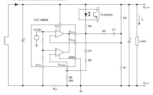
$$V_{OUT} = V_{REF} \times \frac{R1 + R2}{R1} \quad (V)$$
