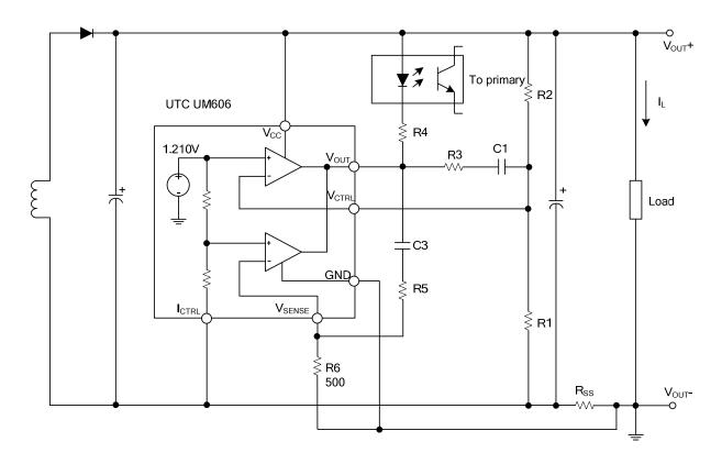
$$\begin{split} V_{OUT} = & \left[ V_{REF} + \left( I_L \times R_{SS} \right) \right] \times \frac{R1 + R2}{R1} - \left( I_L \times R_{SS} \right) \ \, (V) \end{split}$$
