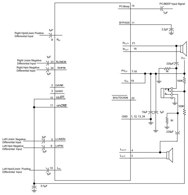
Note: A  $0.1\mu F$  ceramic capacitor must be placed much closely to the IC. For filtering lower frequency noise signals, a larger electrolytic capacitor of  $10\mu F$  or greater should be placed as close as possible to the audio power amplifier.
