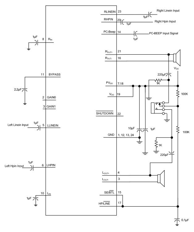
Note:  $1\mu F$  ceramic capacitor should be placed as close as possible to the IC to filter the higher-frequency noise.
