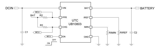
Fig2. Typical Application Circuit Interfacing to a MCU
