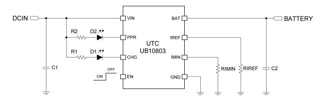
Fig1. Typical Application Circuit for LED Display
