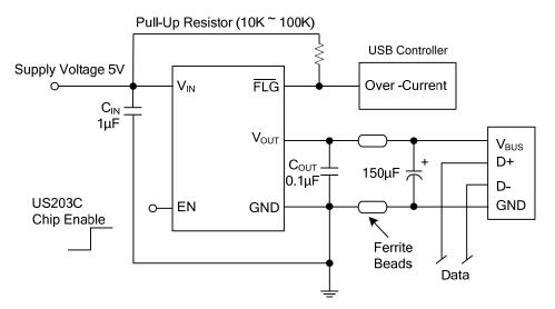
Note: A low-ESR 150 $\mu$ F aluminum electrolytic or tantalum between V<sub>OUT</sub> and GND is strongly recommended to meet the 330mV maximum droop requirement in the hub V<sub>BUS</sub>. (see Application Information Section for further details)
