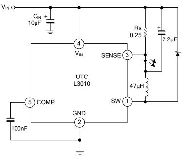
4.5~40V input voltage, 350mA output LED driver
