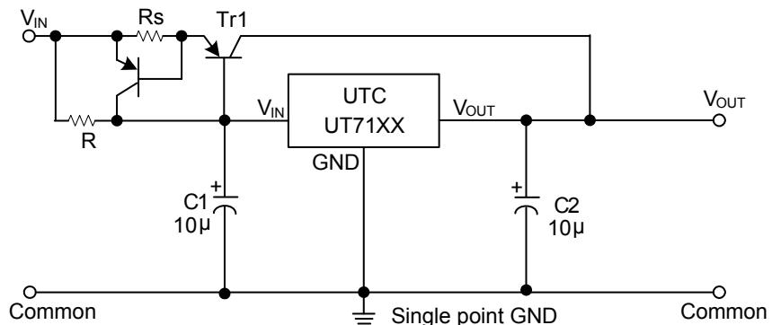
Circuit for increasing output voltage
