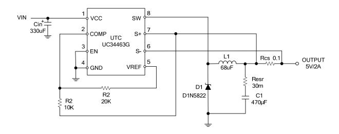
Note: If  $V_{CC}$ >24V, COMP pin to GND need to add 0.1uF (option) compensation capacitor.
