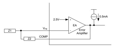
Note: Error amplifier can source or sink up to 0.5mA.
