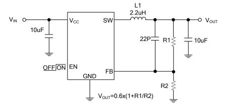
$V_{OUT}=V_{FB} \times (1+R1/R2), V_{FB} = 0.6V, R2 suggest 60k^300k\Omega$
