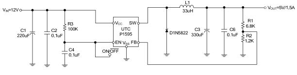
$$V_{OUT} = V_{FB} \times \left(1 + \frac{R1}{R2}\right), V_{FB} = 0.75V. R2 = 0.75K \sim 4K$$
