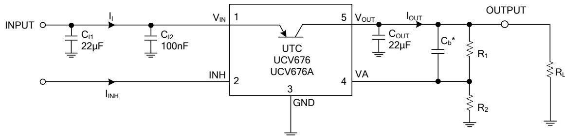
$$V_{OUT} = [(R_1 + R_2) \times V_{REF}] / R_2$$
