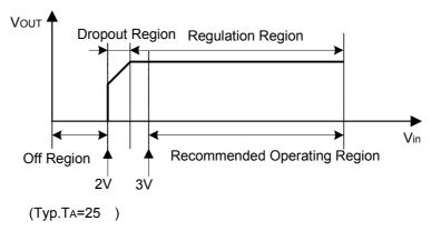
For proper regulation, this device must be operated in the Recommended Operating Region shown above.
