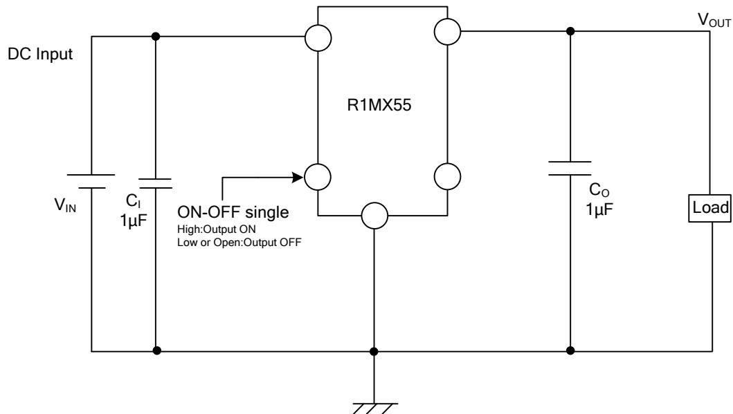
■ ELECTRICAL CHARACTERISTICS MEASURING CIRCUIT(FOR SOT-89-5)
