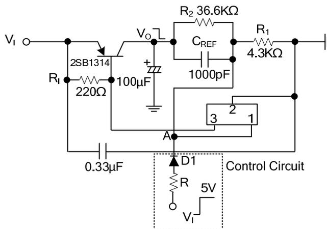
Set control circuit resistor R so that voltage of point A is more than 1.5V and less than 5V
