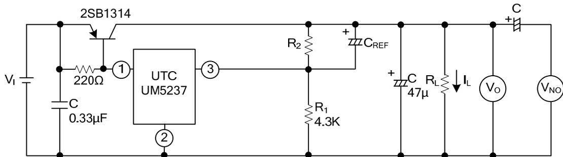
(b) Ripple rejection test circuit
