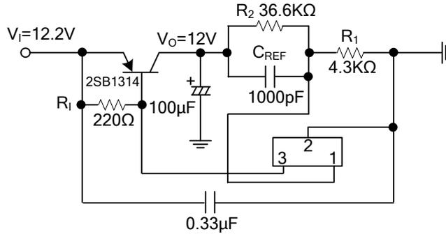
$$V_O = V_{REF} \times \left( 1 + \frac{R_2}{R_1} \right) V, \quad V_{REF} = 1.26V$$
