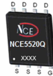
DFN3X3 EP top view
