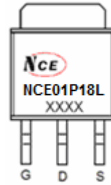
Marking and pin assignment
