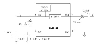
Figure 2 Input DC Coupling Output AC Coupling
