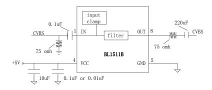
Figure 1 AC Coupling Application Schematic
