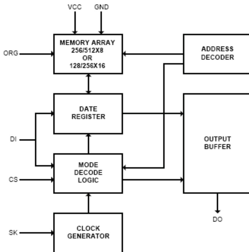
Notes: When the ORG pin is connected to VCC, the "x 16" organization is selected. When it is connected to ground, the "x 8" organization is selected. If the ORG pin is left unconnected and the application does not load the input beyond the capability of the internal 1 Meg ohm pullup, then the "x 16" organization is selected.
