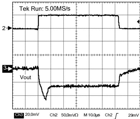
$V_{OUT}=2.5\text{V}$ ,  $I_{OUT}=0\sim 50\text{mA}$ , no  $C_{IN}$ ,  $C_{OUT}=10\mu\text{F}$ ,  $t_s=t_r=2\text{ns}$
