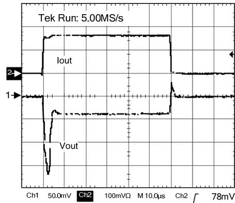
$V_{OUT}=2.5\text{V}$ ,  $I_{OUT}=50\text{mA}$ , no  $C_{IN}$ ,  $C_{OUT}=4.7\mu\text{F}$ ,  $t_s=t_r=20\text{ns}$
