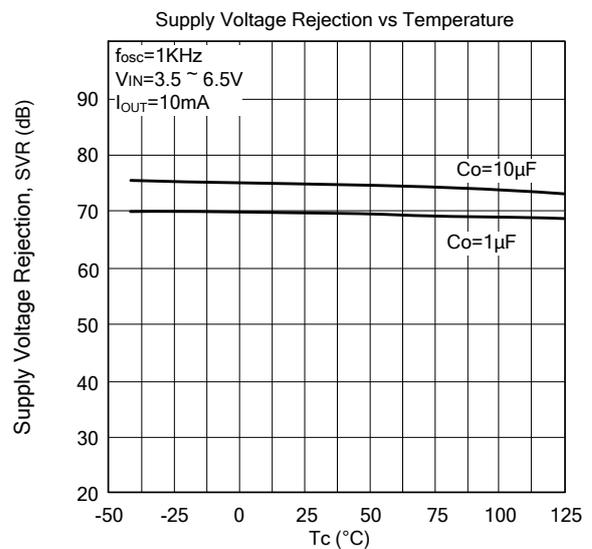
■ TYPICAL CHARACTERISTICS(Cont.) ( $T_J=25^{\circ}\text{C}$ ,  $C_I=1\mu\text{F}$ ,  $C_O=2.2\mu\text{F}$ ,  $C_{BYP}=100\text{nF}$ )
