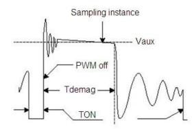
Fig.2: Auxiliary voltage waveform
