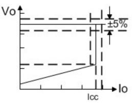
Fig.1 : Typical CC/CV curve
