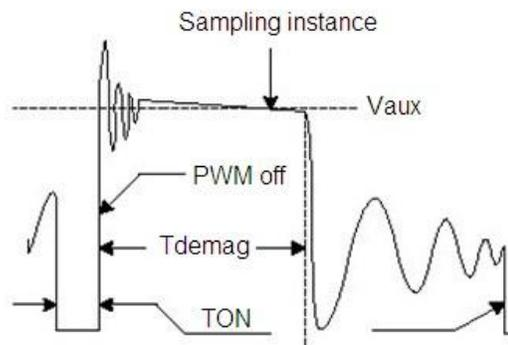
Fig.2: Auxiliary voltage waveform
