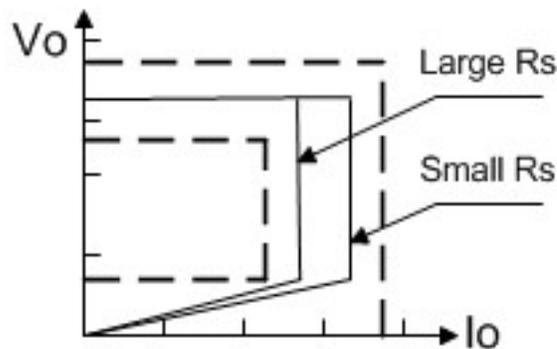
Fig.3: Adjustable output power by changing
