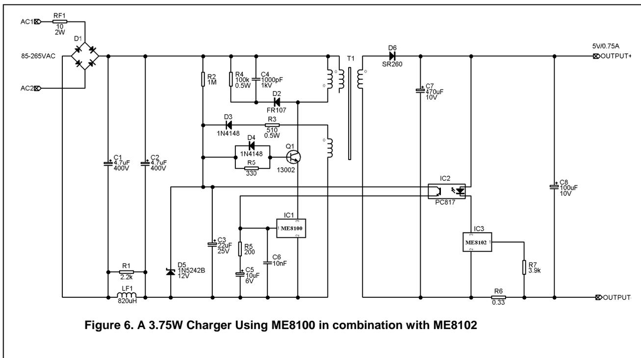
**Figure 6. A 3.75W Charger Using ME8100 in combination with ME8102**
