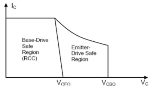
**Figure 5. NPN Reverse Bias Safe Operation Area**
