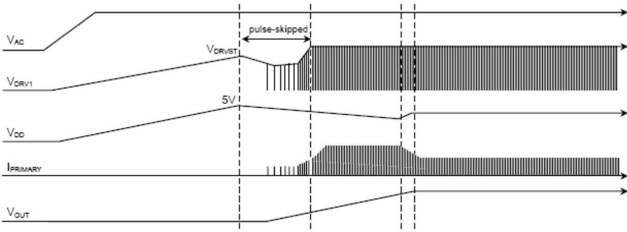
**Figure 3. Startup Waveforms**
